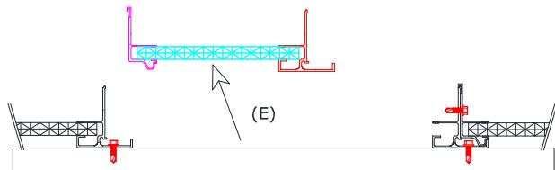
4 - A lug profile is installed on the module of substitution (F). In first, install the module of substitution
