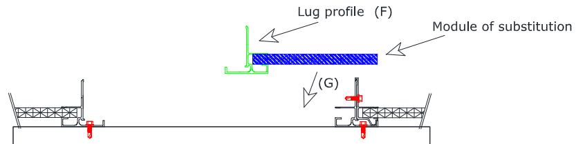
5 - Fix the module of substitution (H), replace the lug profile of the module in good condition by a socket profile (I) and install it (J)
